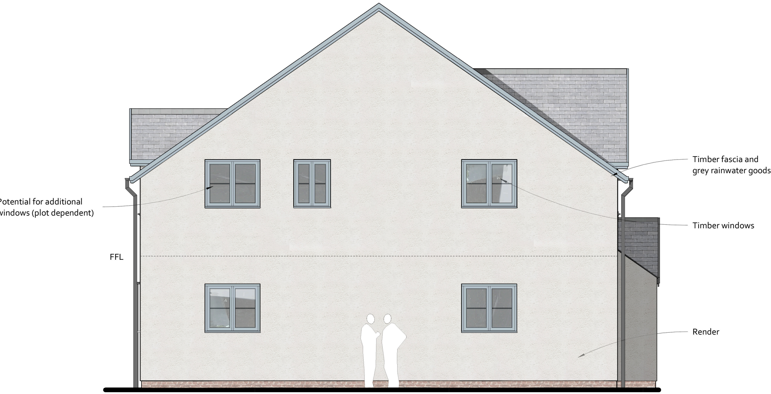
Side Elevation B 1 : 50
