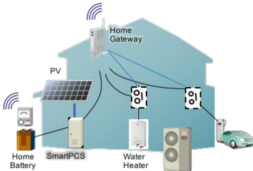
Figure 5.1.1: Example of DR-capable technologies that can be installed in a house or cottage
