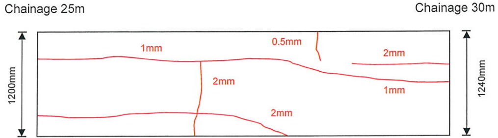
Figure 9: Wall Height, Crack Locations and Sizes for Chainages 25m to 30m
