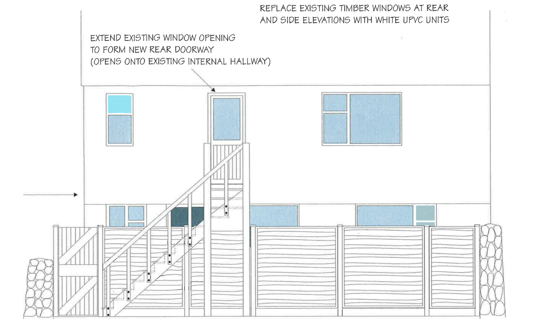
EXISTING GARDEN WALL PROPOSED EXTERNAL OPEN TREAD STAIRS, FROM EXISTING CONCRETE PATIO TO DOOR AT FIRST FLOOR 2 METRE HIGH PANEL FENCE ALONG EXISTING CONCRETE PATIO EXISTING GARDEN WALL
