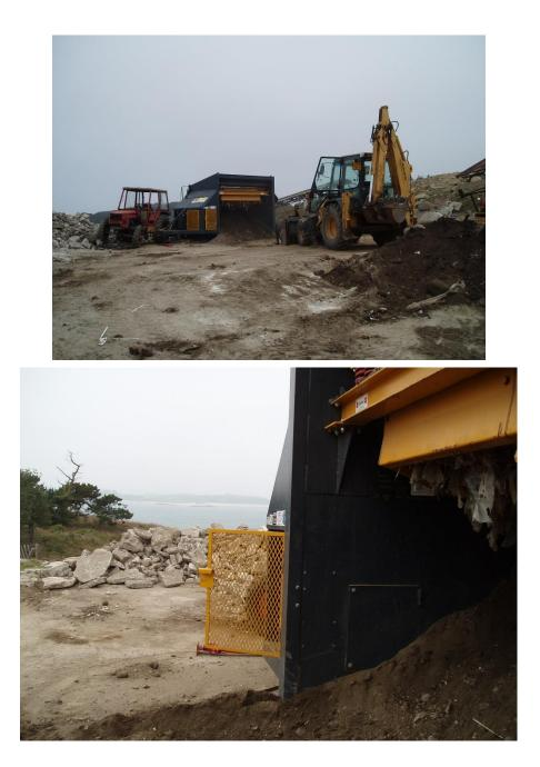
• Output is enhanced: The new rotary trommel is used to provide different grades of bagged recycled aggregates after crushing and screening (left) and the new conveyor is integrated with the new screen (right)
