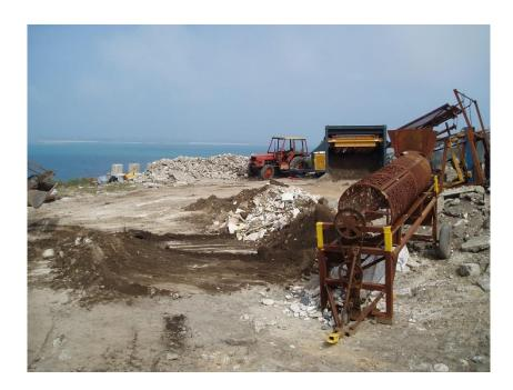
In the photo below, the whole system is integrated on the middle tier at Pendrethen, producing quality recycled aggregates from imported C&D waste streams and reselling to local markets.
