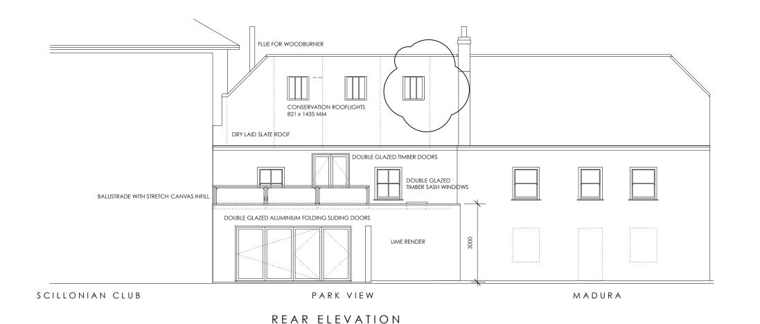
REVISION A 30.11.15 chimney stack removed. rooflight to rear elevation
