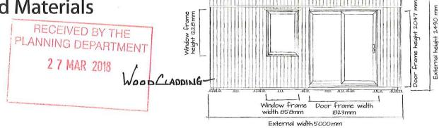
Use a flat level base allowing 100mm all around in addition to external cabin measurements.
