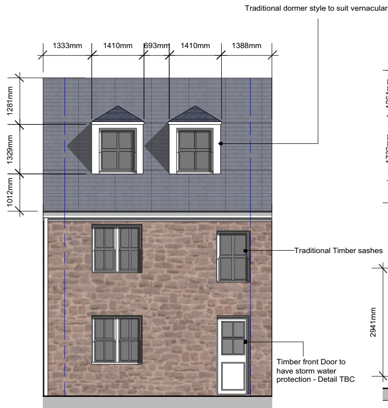
Proposed North Elevation Scale: 1:100
