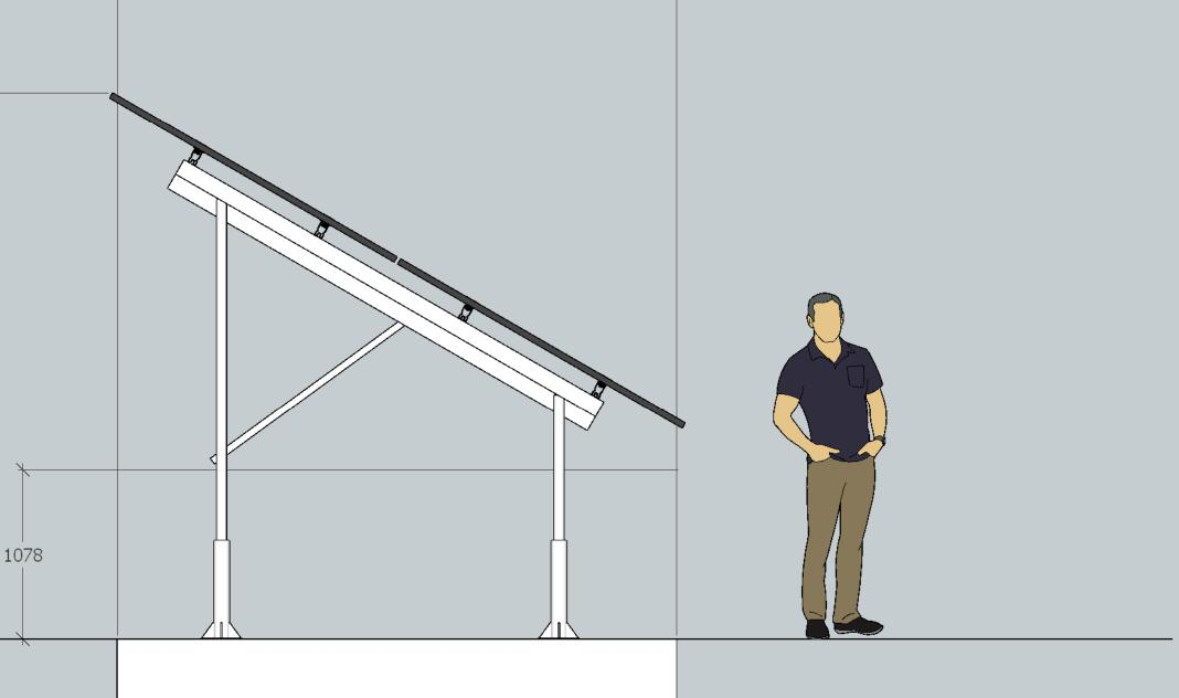
Due to variations in terrain, level of concrete footing above ground will vary depending on location. Height of tables is adjustable. Tables are shown adjusted to maximum height
