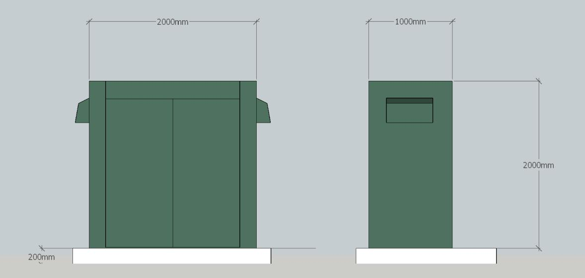
Green cabinet housing WPD Point of Connection, isolation, cable protection and metering equipment. GRP construction, Green (RAL 14 C 39) gloss finish. Mounted on concrete plinth
