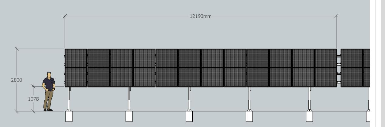
Elevation shows dimensions of one 'Table'. Solar Garden comprises three rows of tables. Due to variations in terrain, level of concrete footing above ground will differ depending on location. Height of tables is adjustable. Tables are shown adjusted to maximum height
