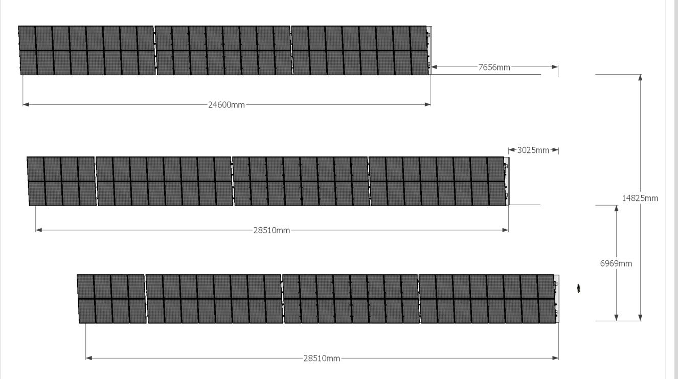
Note: Array spacing takes account of increase in slope as terrain falls away to the North.
