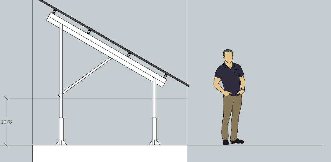
Due to variations in terrain, level of concrete footing above ground will vary depending on location. Height of tables is adjustable. Tables are shown adjusted to maximum height
