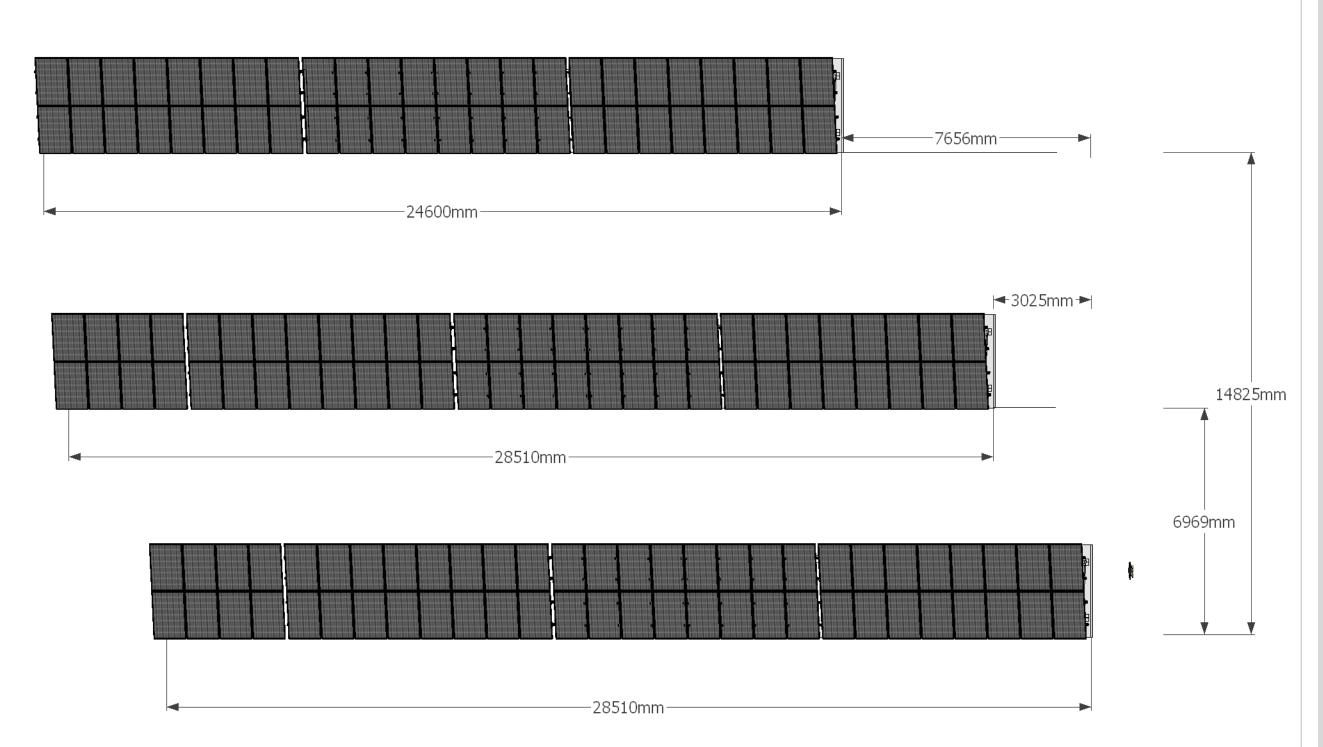
Note: Array spacing takes account of increase in slope as terrain falls away to the North.
