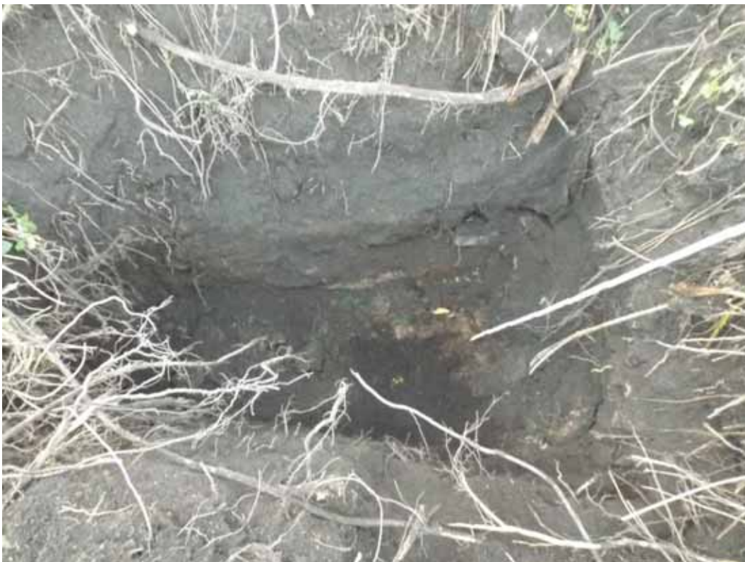
Plate 12: Geotechnical test-pit at north-east end of garden area. There is a single homogenous layer of dark garden soil lying above the ram, the weathered top of the underlying granite.
