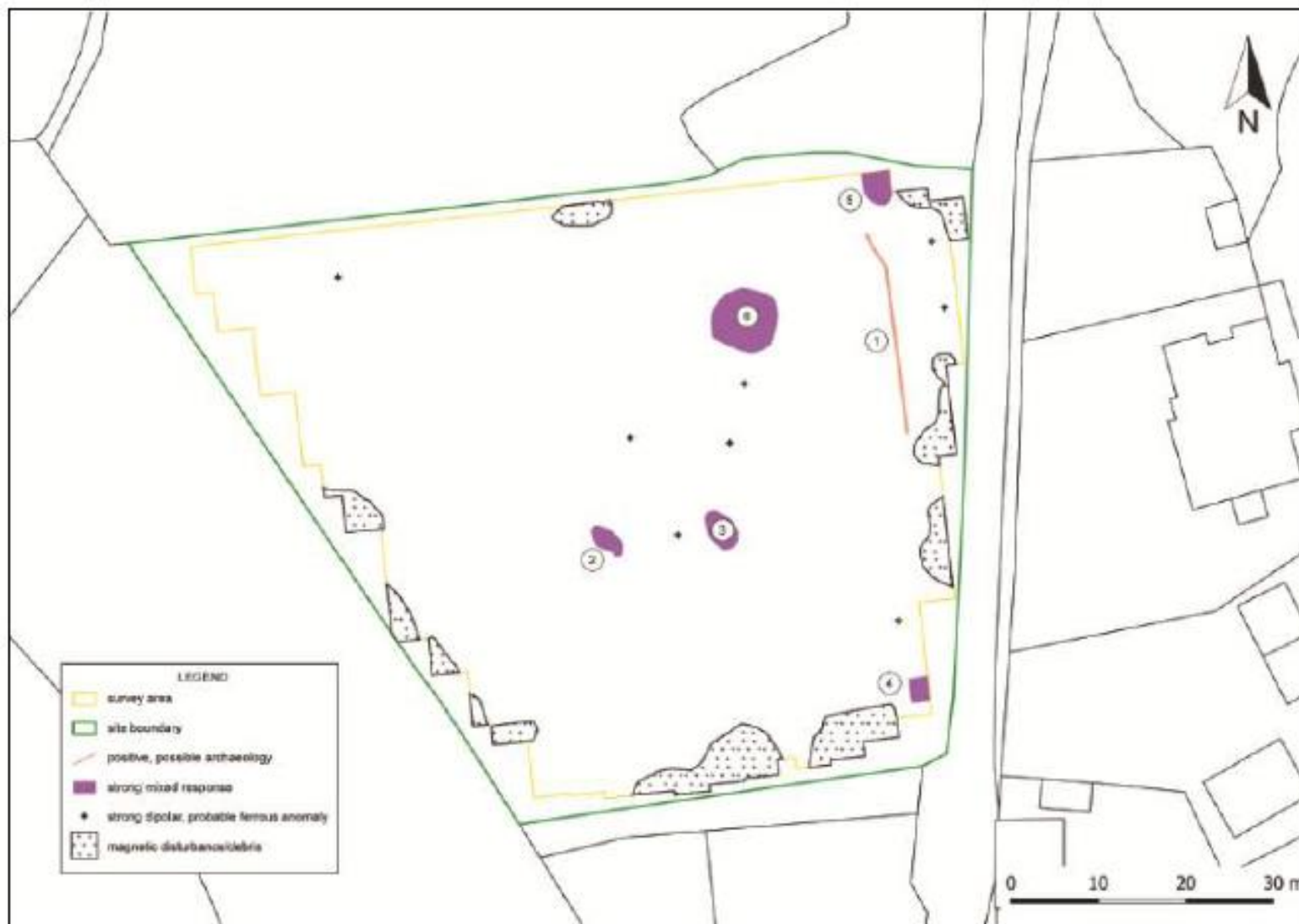
Fig 3 Surveyor's plan presenting interpretation of gradiometer survey data, with numbered anomalies.
