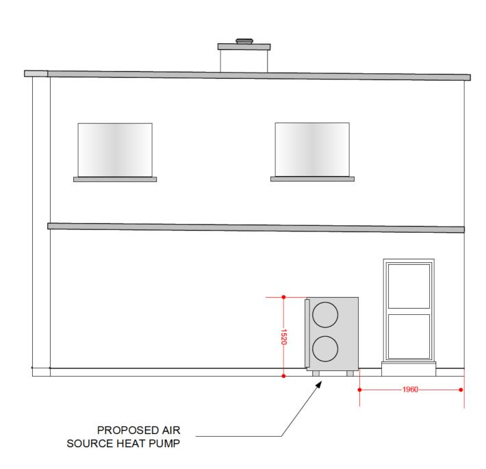
PLAN (PARTIAL) SHOWING POSITIONING OF ASHP
