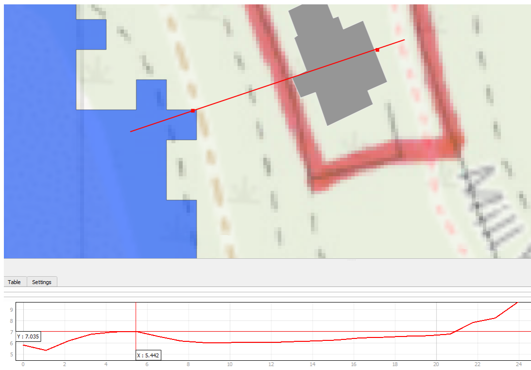
Figure 5: Section through defence and site as indicated.
