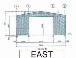
AGRICULTURAL BUILDING 10m x 10m x 4m TO EAVES 6 MAIN STANCHIONS 6 MAIN RAFTERS 1 GABLE STANCHION 2 ROLLER SHUTTER DOOR POSTS 2 DIAGONAL ROOF BRACES 2 DIAGONAL ROOF BRACES
