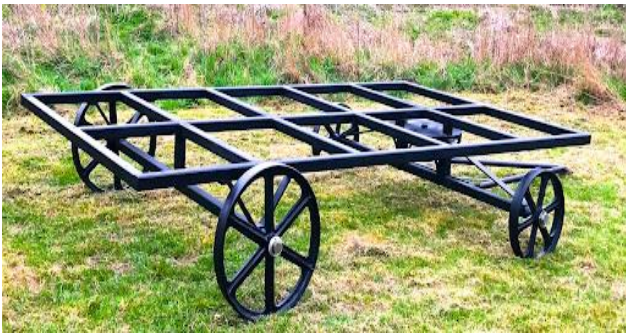
Typical chassis construction for the shepherd’s huts. Steel framed and steel wheels, coated, primed, undercoat and painted black in colour.
