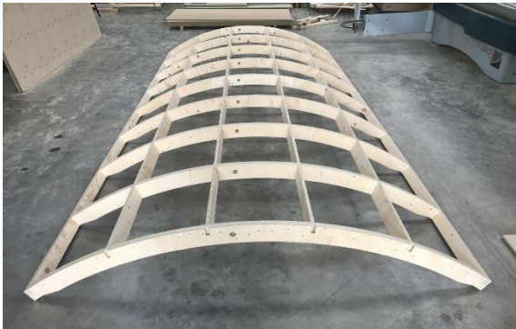
Typical carcass construction showing floor and ribs mounted a chassis and the basic form and structure of the roof curvature.
