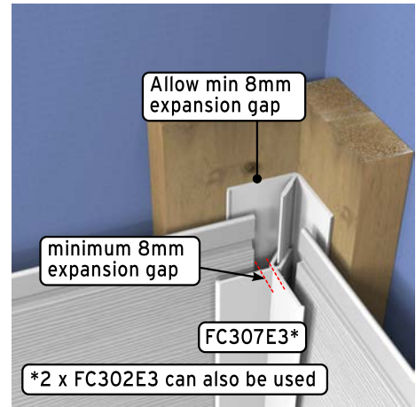
Typical Internal Corner
