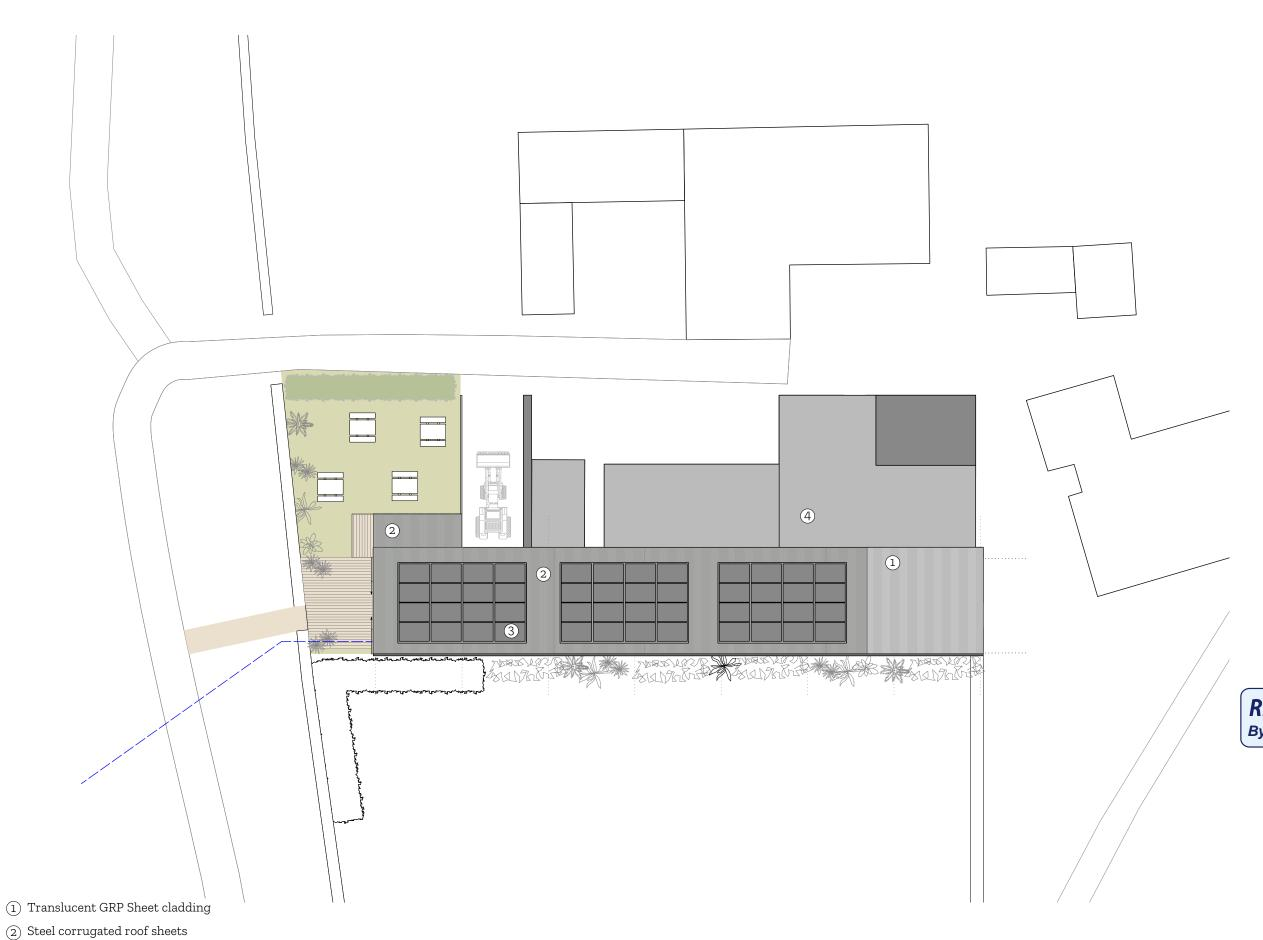
3 Photovoltaic Panels (4) Existing metal roofs ARBOR
