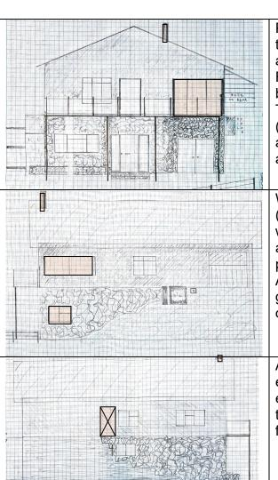
Proposed front elevation: removal of the existing timber balcony that wraps around the front and to the south side. Replacement with simple front balcony with glazed balustrade. The RHS window is removed (currently a bow or bay style window) and replaced with sliding doors, to access the balcony
