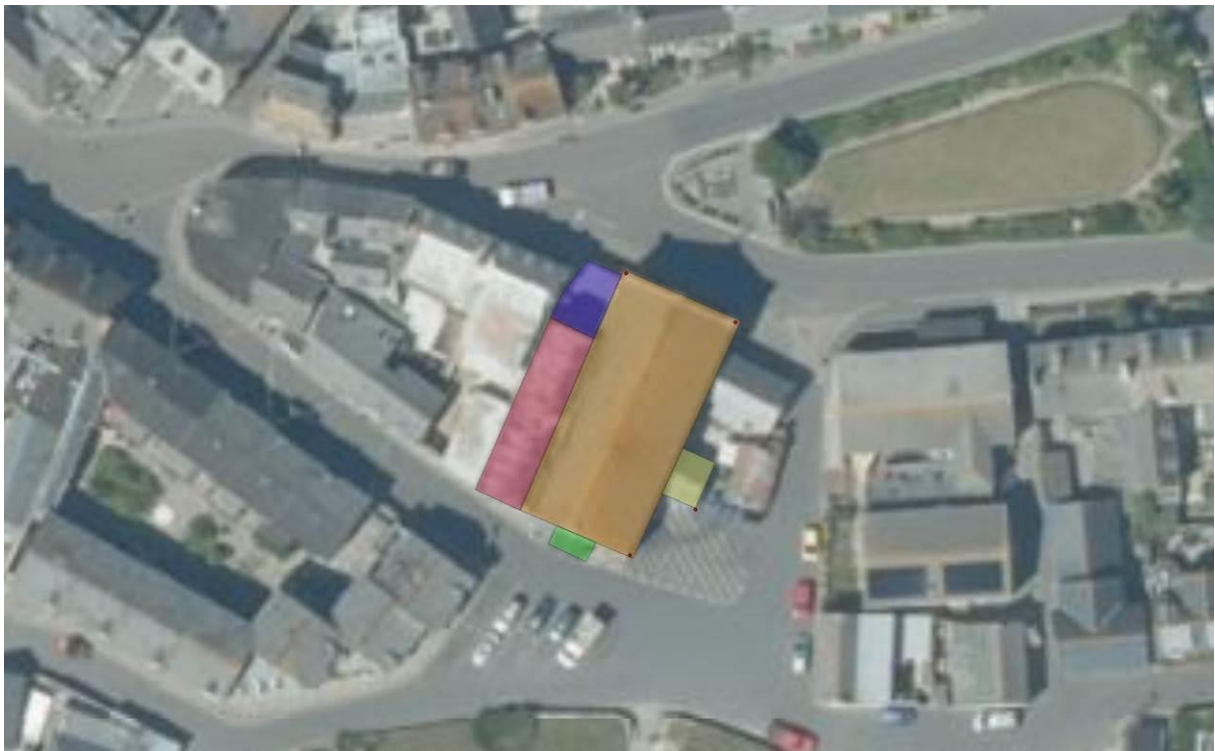
Map 02 – Showing the main hall (orange), 1970’s extension (pink); front porch (purple); rear porch (green) and plant room (yellow).
