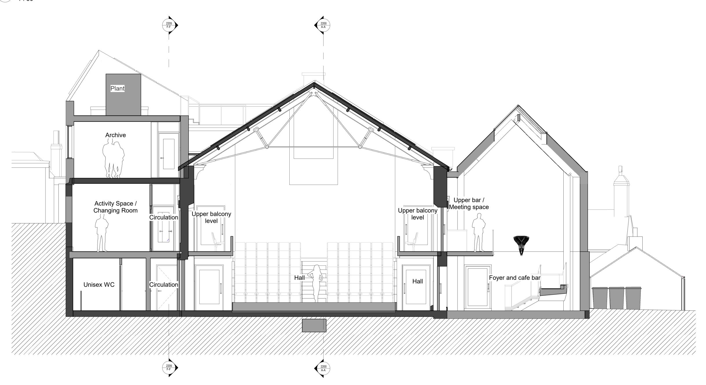
For the comparative existing section following the same line see: Section BB – Existing, drawing number 241601-PUR-01-ZZ-A-1201
