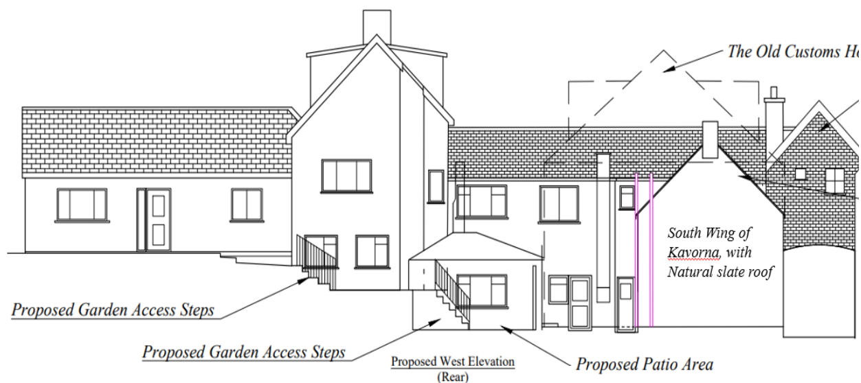
Fig. 18: Drawing of the rear, south-west elevation of Kavorna, with location of the south wing (Paul Osborne).
