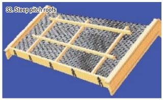
On roofs with a pitch steeper than 20°, a free-standing timber framework must be constructed and rested against the front (eaves) edging board. This helps prevent soil slippage.
