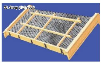
On roofs with a pitch steeper than  $20^\circ$ , a free-standing timber framework must be constructed and rested against the front (eaves) edging board. This helps prevent soil slippage.
