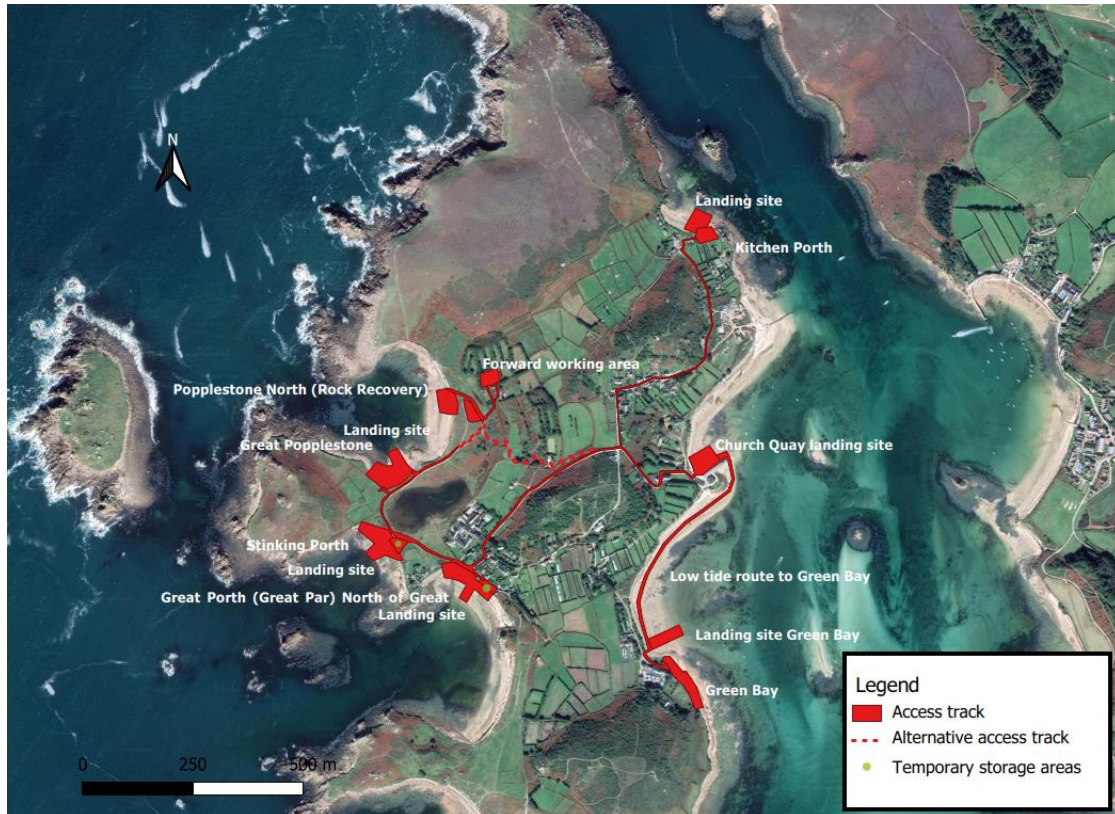
Figure 20: Construction access routes across the island of Bryher.
