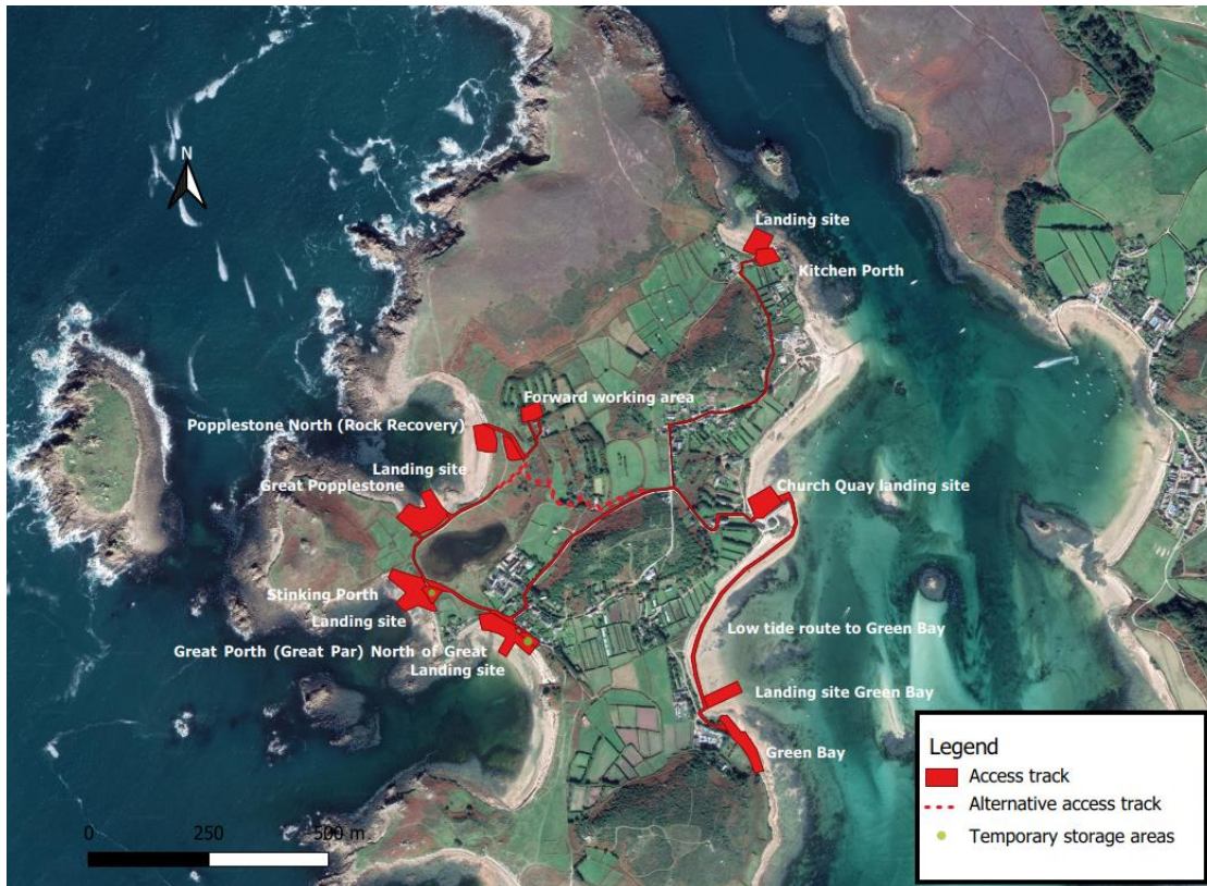
Figure 2-28: Construction access routes across the island of Bryher
