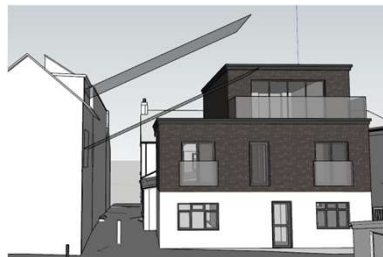
3D images demonstrating 25* rule of thumb test is passed & overlooking from proposed extension is minimal
