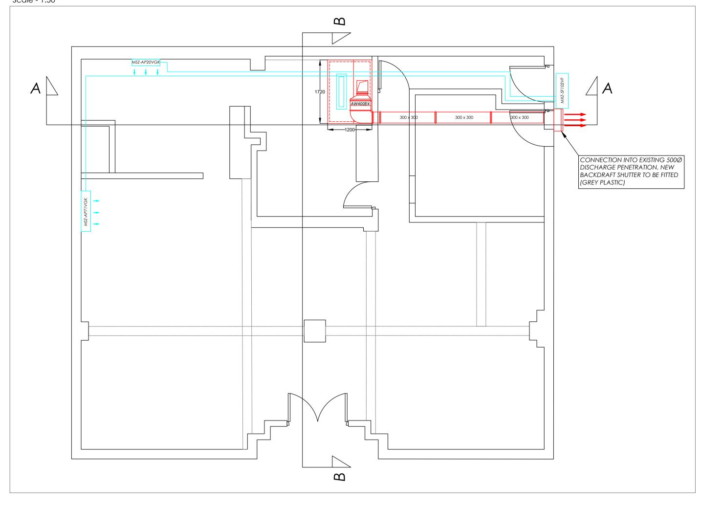
PLEASE NOTE THAT WHILST WE HAVE NOT INCLUDED A MECHANICAL FRESH AIR SUPPLY INTO THE KITCHEN, IT IS RECOMMENDED THAT THIS BE INSTALLED WITH ANY SYSTEM EXTRACTING AIR FROM A ROOM
