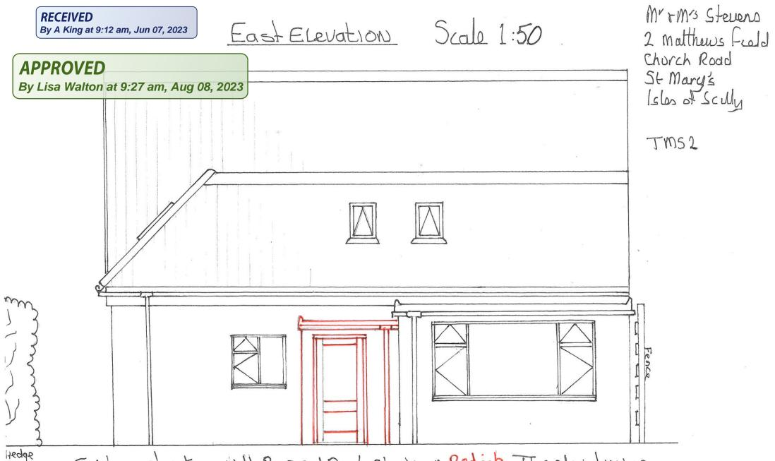
Existing elevation with Proposed Porch shown in Red ink. This elevation is the same without the Porch as the existing back door currently occupies the same relative Position - it is Just 1.8 m Further back. See: ground floor Plan.
