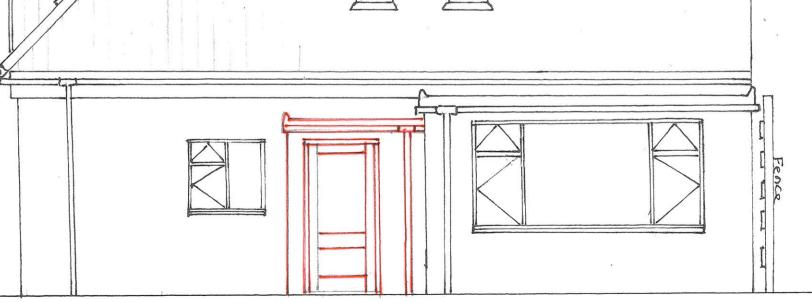
Hedge Existing elevation with Proposed Porch shown in Red ink. This elevation is the same without the Porch as the existing back door currently occupies the same relative Position-it is Just 1.8 m further back. See: ground floor Plan.
