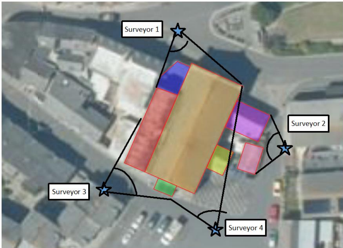
Map 02 – showing surveyor positions around the building. The different elements of the building are identified by different colours - the main hall (orange), 1970's extension (red); front porch (blue); rear porch (green), plant room (yellow), cottage (dark purple) and stone shed (light pink).
