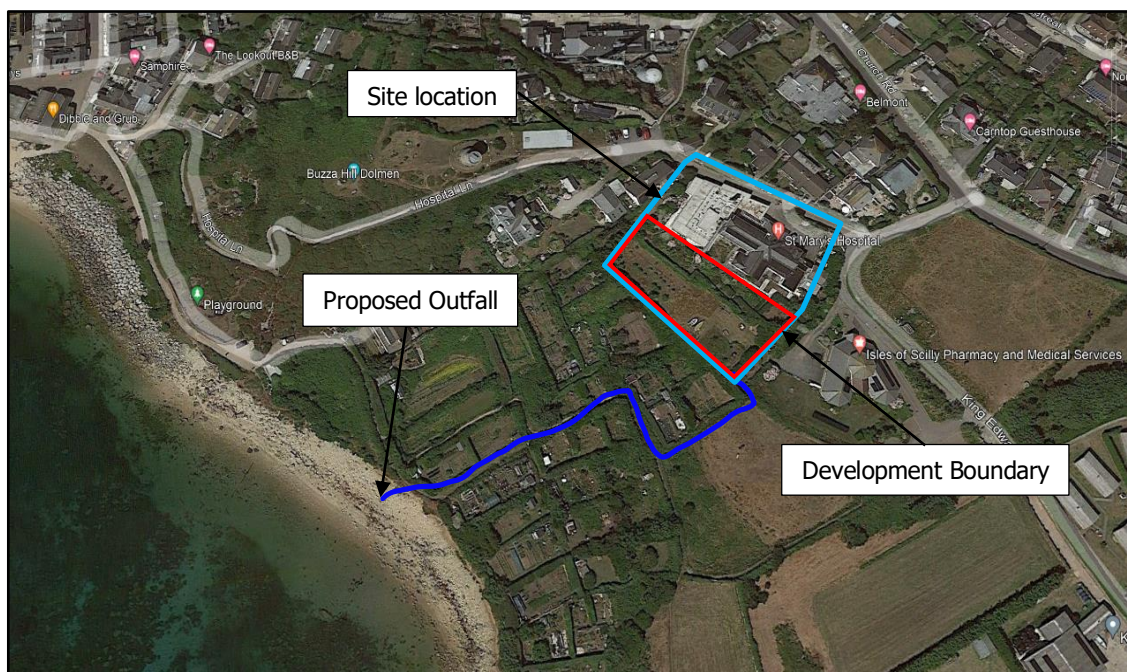
Figure 4 – Indicative Location of Surface Water Outfall
