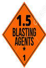
Subclass 1.5: An insensitive substance with a mass explosion hazard
