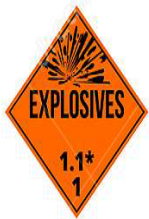
Subclass 1.1: Explosives with a mass explosion hazard
